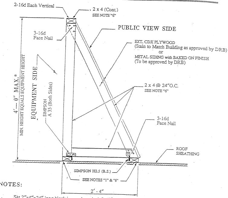
Set 2"x4"x24" long block in mastic typical @ 48" O.C. Attach each block to purlins or subpurlins with 2-3/8" Dia. x 5" lag bolts. Seal head of lag bolt with mastic. Weatherproofing of existing roofing is to be maintained.
