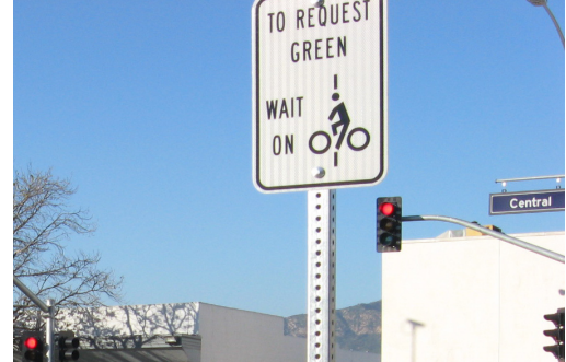
Figure 5-17. Bicycle detection sign at Maple and Central
