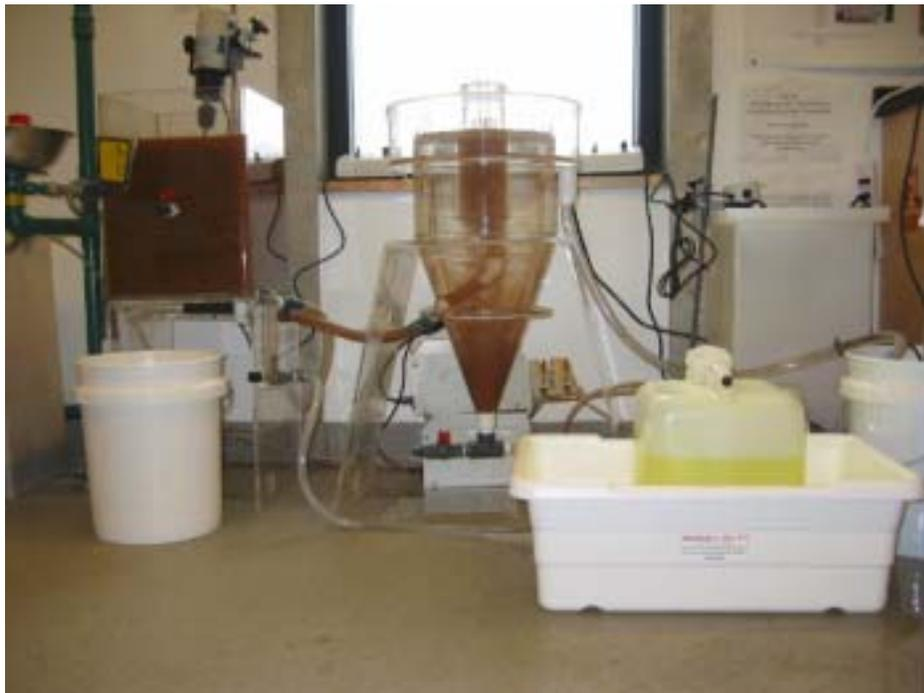
**Figure 3.9** Small-scale MIEX<sup>®</sup> pilot unit
