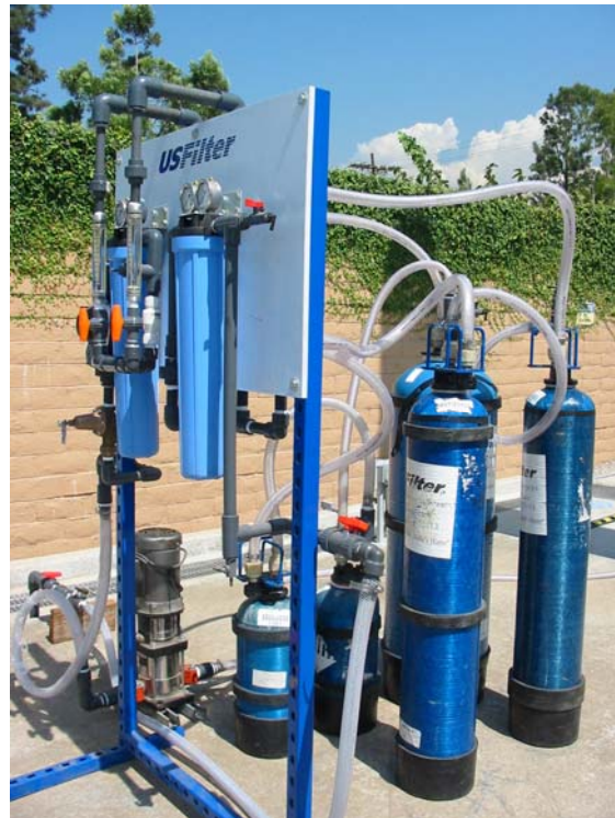
USF/R&H SBA Pilot Unit (lead-lag canisters in the foreground)
