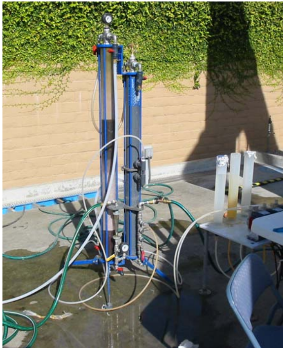
Filtration Reduction/Filtration System (reduction column on right, filter on left; chemical addition from cylinders on table)
