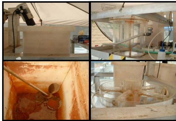
MIEX Phase A testing – System components shown include reactor and settler.
