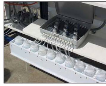
A flow-paced chromium spiking system was used to deliver 100 µg/L hexavalent chromium to the influent groundwater source (left) that was used in the pilot units. Parallel lead/lag pilot-scale trains of strong base (two large canisters) and weak base (small canisters) anion exchange resin were used for the study (second from left). Ion exchange columns tested strong-base anion exchange with brine regeneration and recycle (second from right). An autosampler was used to collect samples from the ion exchange skid to capture chromatographic peaking (right).
