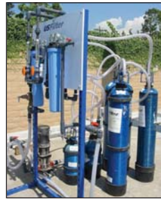
A flow-paced chromium spiking system was used to deliver 100 µg/L hexavalent chromium to the influent groundwater source (left) that was used in the pilot units. Parallel lead/lag pilot-scale trains of strong base (two large canisters) and weak base (small canisters) anion exchange resin were used for the study (second from left). Ion exchange columns tested strong-base anion exchange with brine regeneration and recycle (second from right). An autosampler was used to collect samples from the ion exchange skid to capture chromatographic peaking (right).
