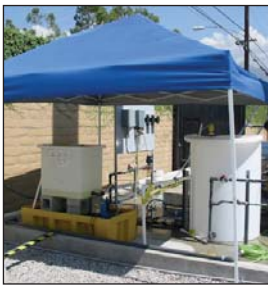
A flow-paced chromium spiking system was used to deliver 100 µg/L hexavalent chromium to the influent groundwater source (left) that was used in the pilot units. Parallel lead/lag pilot-scale trains of strong base (two large canisters) and weak base (small canisters) anion exchange resin were used for the study (second from left). Ion exchange columns tested strong-base anion exchange with brine regeneration and recycle (second from right). An autosampler was used to collect samples from the ion exchange skid to capture chromatographic peaking (right).
