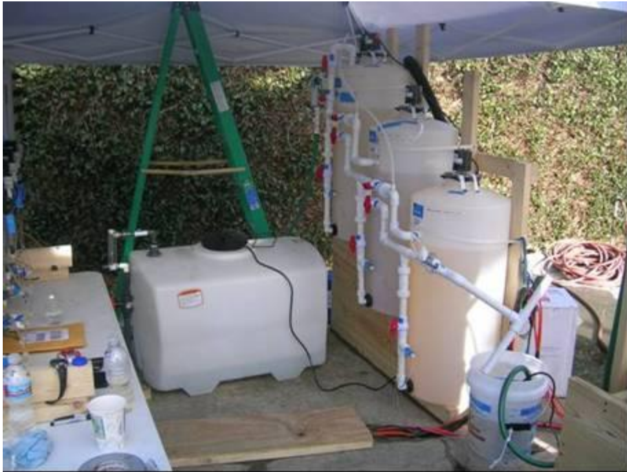
Figure B-4. Three Aeration Columns in Series and Rapid Mix Tank
