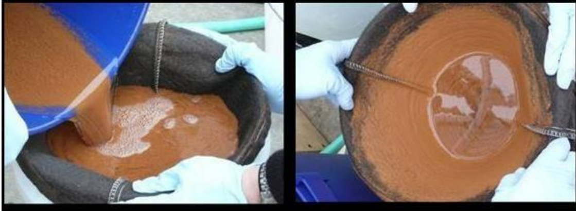
Figure 5-16: Flo-Trend Solids Separation of Backwash Water Solids
