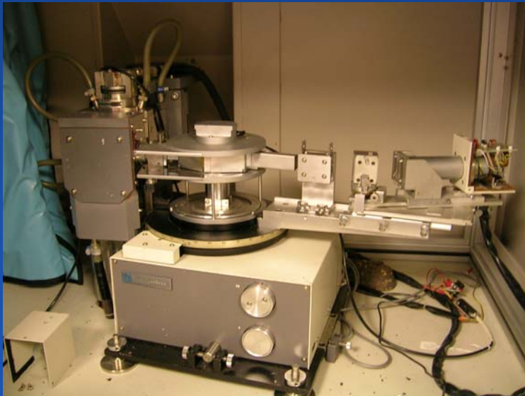
Rigaku 300 diffractometer with rotating copper anode
