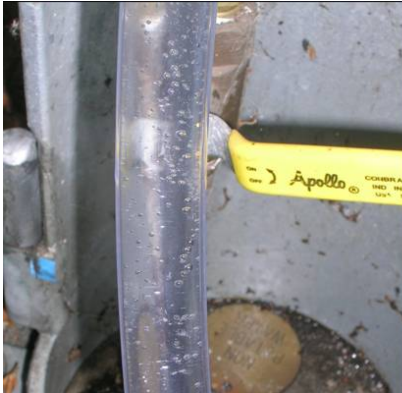
Figure 3: Release of some supersaturated CO 2 in the sampling line
