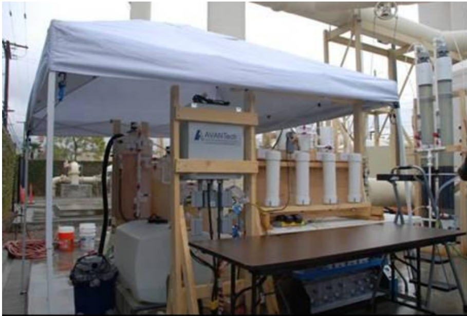
Figure B-2. Chemical Feed Day Tanks (White PVC columns)
