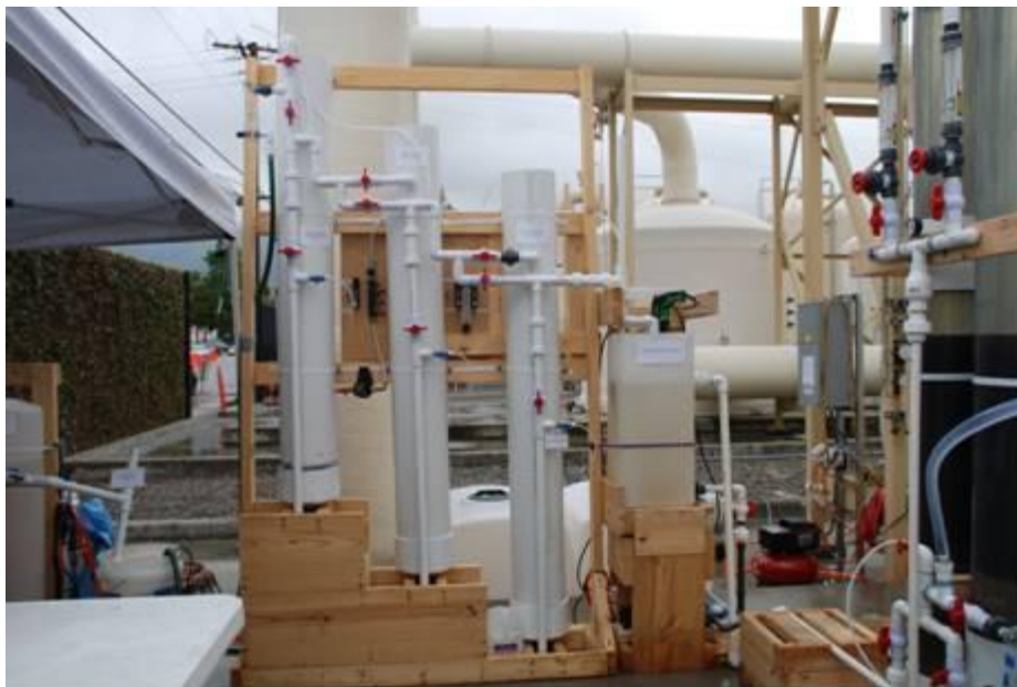
Figure B-4. Three Aeration Columns in Series and Rapid Mix Tank
