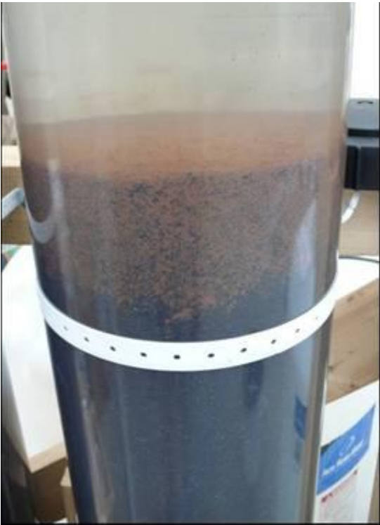
Figure B-8. Start of Filter Backwashing (Overflow of backwash water)
