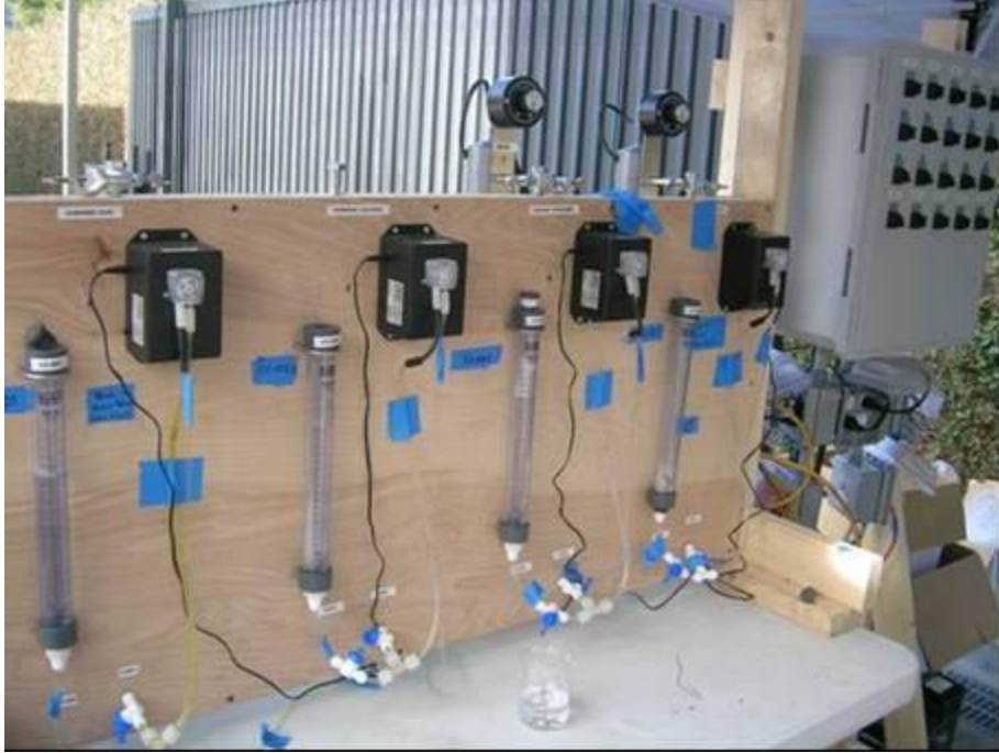
Figure B-2. Chemical Feed Day Tanks (White PVC columns)
