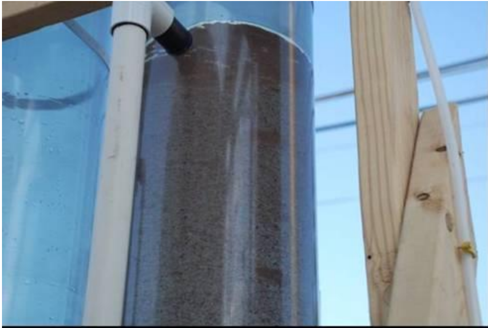
Figure B-9. End of Filter Backwashing (Overflow of backwash water)
