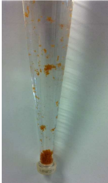
Figure 5-9. Settled Solids in Imhoff Cone for Glendale Water Sample with Fe:Cr(VI) of 34:1
