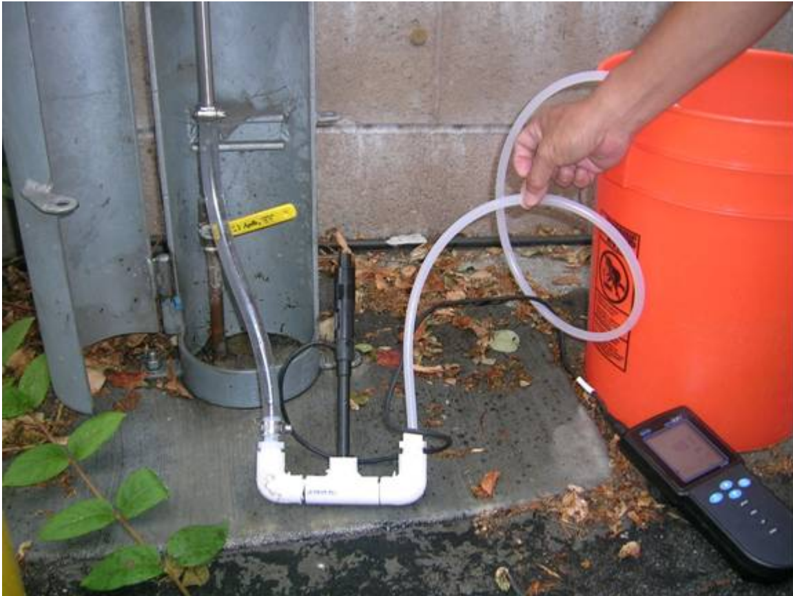
Figure 2: pH and temperature measurement with the specialized sampling apparatus developed to minimize CO 2 off gassing (pH probe shown in the center of the apparatus)
