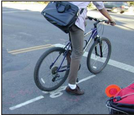
Figure 8-30: Bicycle Loop Detector Marking
