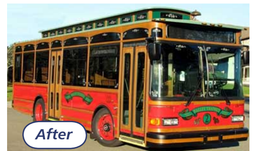
BELOW: Cable Car Classics conversion of a 30’ low floor Gillig Phantom bus.
