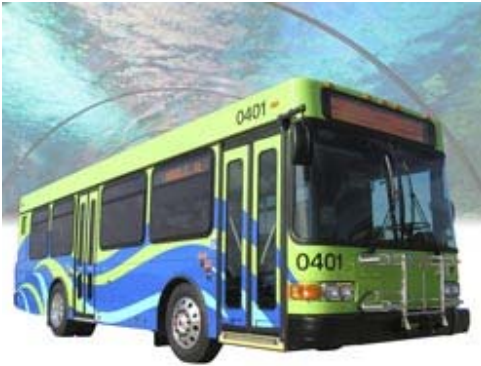
BELOW: Gillig low floor hybrid electric 30' conventional bus.
