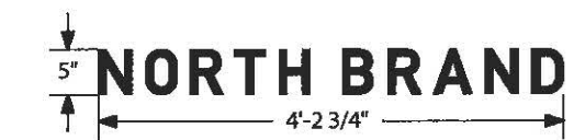
2 DETAIL BUILDING ID- NORTH BRANDf Scale: 3/4" = 1'-0"
