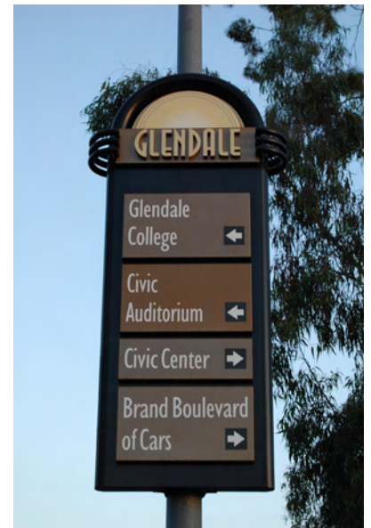
Signs from this thematically designed program are difficult for drivers to read.
