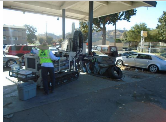
Photograph 10: View of the soil sampling activities at soil boring location SB11.
