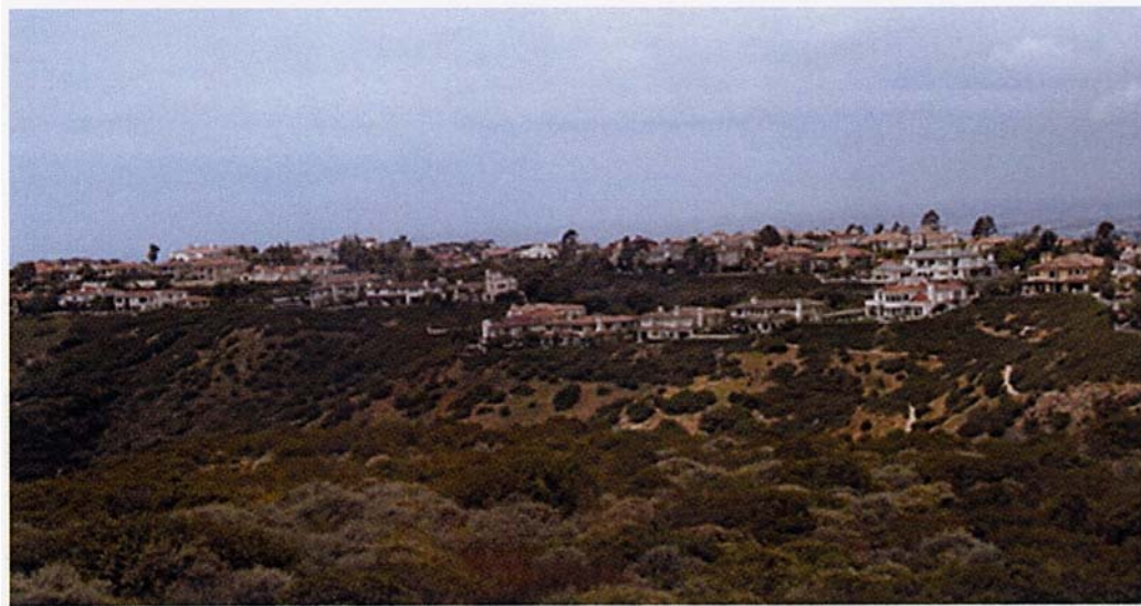
Figure 4-4: Example of Vegetation Management at the Urban-Wildland Interface (Residential community in southern California that uses fuel modification to reduce its fire hazard. Note selective thinning of vegetation in the slope below the structures. Closer to the structures, there is a zone of fire-resistive ornamental plants that are irrigated. The vegetation in the foreground is in its natural state.)
