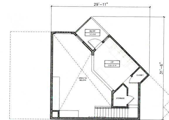
UNIT B3-L2 2 BEDROOM - 2 BATH LOFT LIVABLE AREA: 130 SQ. FT. LOFT BUILDABLE AREA: 251 SQ. FT. BALCONY: 50 SQ. FT.
