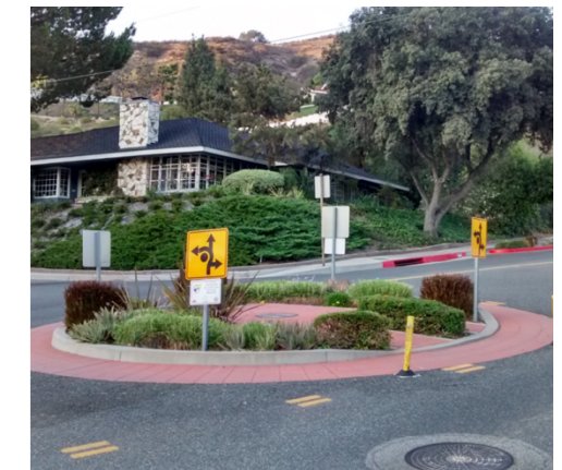
Traffic calming elements, such as traffic circles at neighborhood street intersections, help to reduce auto travel speeds.
