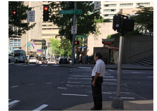
No-right-turn-on-red policies in downtown Seattle help reduce conflicts between drivers and pedestrians.
