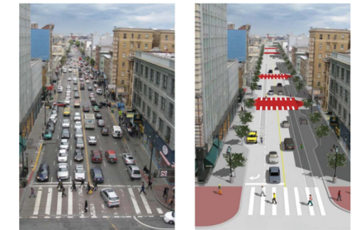
Street design to ensure safe travel behavior is supported by traffic calming measures on arterial streets. Image Source: People for Bikes
