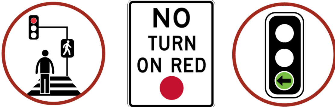
Figure 6-4 Pedestrian Head Starts, Protected Left-Turn Phases, and No Right Turns on Red Reduce Driver/Pedestrian Conflicts
