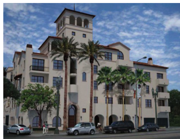
ABOVE: Roofline modulation can create the appearance of distinct buildings in a single massing while minimizing building scale.
