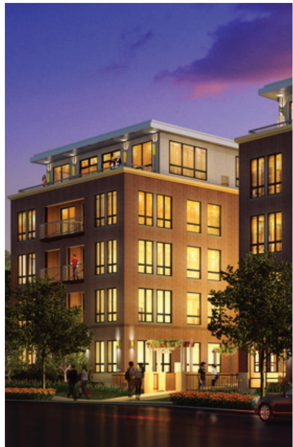
ABOVE: An upper level stepback can reduce the scale and massing of a building, while reinforcing the pedestrian scale of the public realm.
