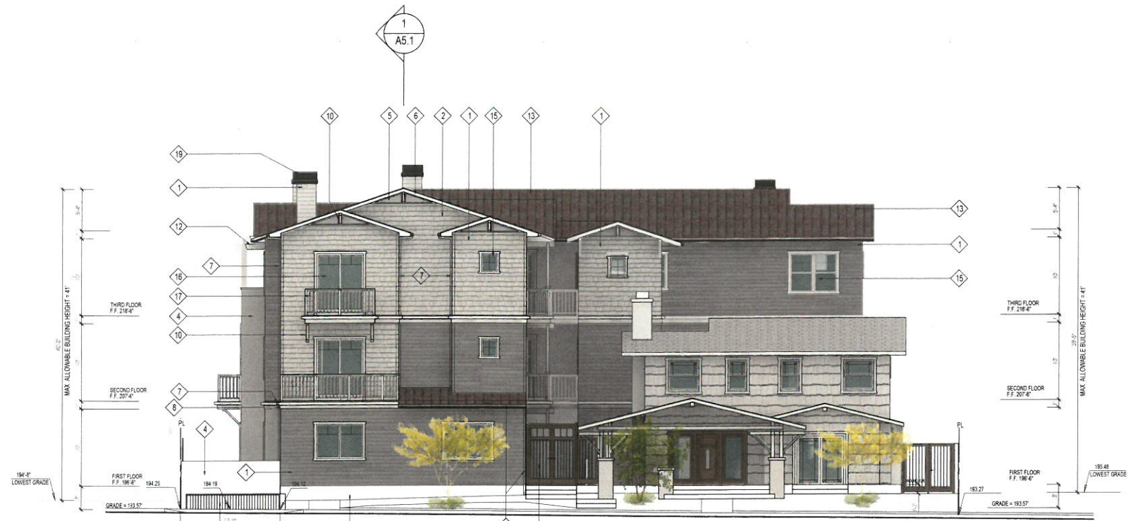
1 BUILDING WEST ELEVATION SCALE 1/8"=1'-0"
