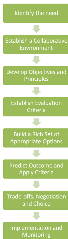
Figure 4 – Eight-step station access planning flowchart
