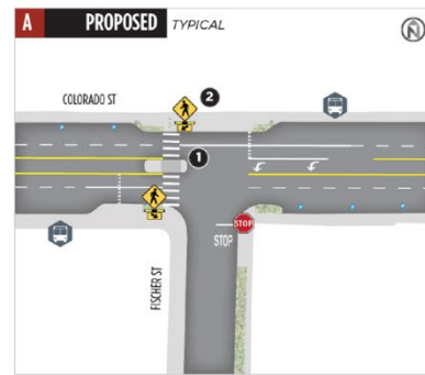
1 Upgrade marked ladder crossing to median refuge island 2 Replace existing circular flashing beacon system with rectangular rapid flashing beacons (RRFB)
