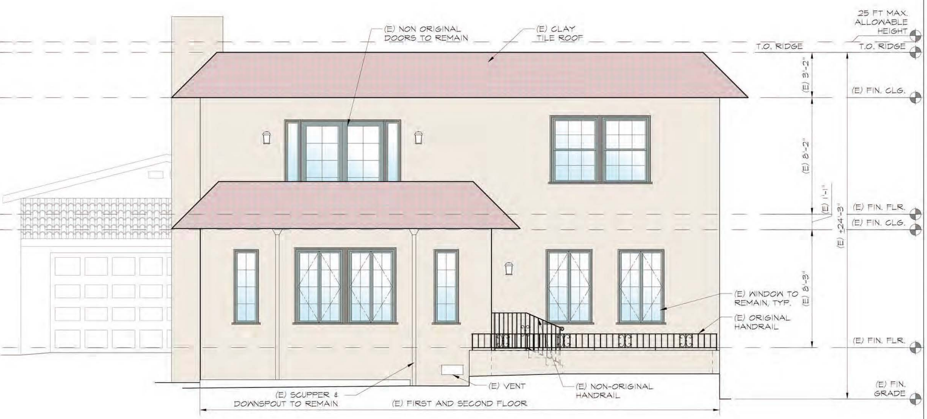
2 Proposed West Elevation Scale: 1/4" = 1'-0"
