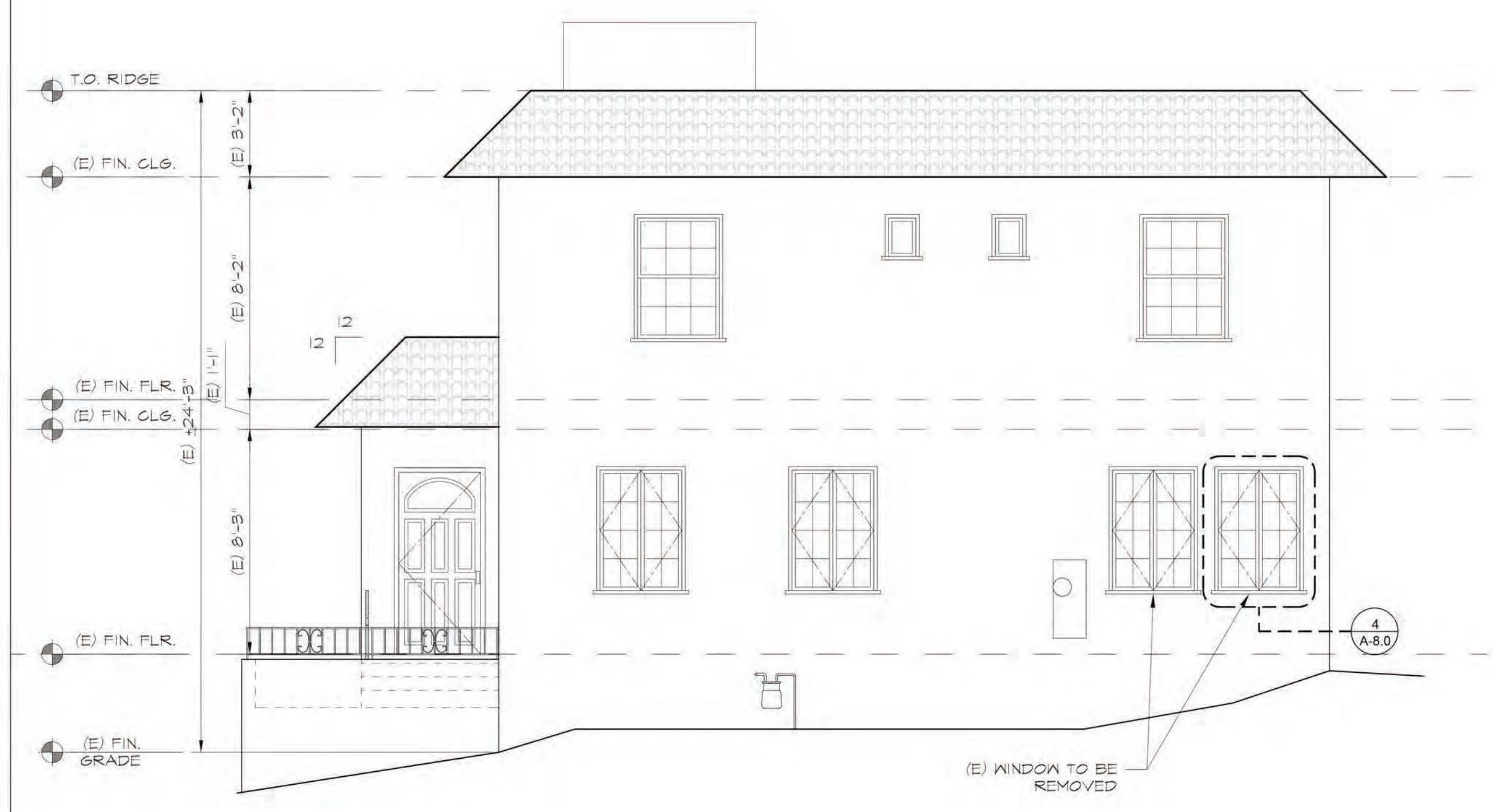
3 Existing South Elevation Scale: 1/4" = 1'-0"
