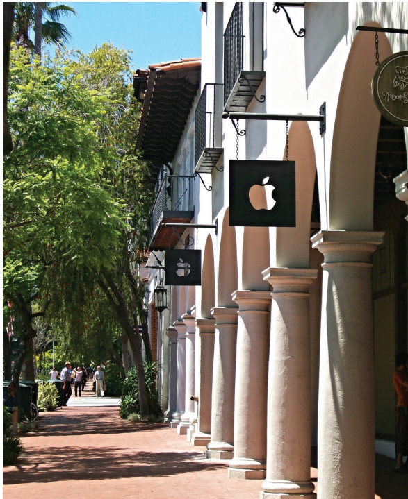
ABOVE: Laser cut projecting signs identify businesses and add an architectural design element to the building.
