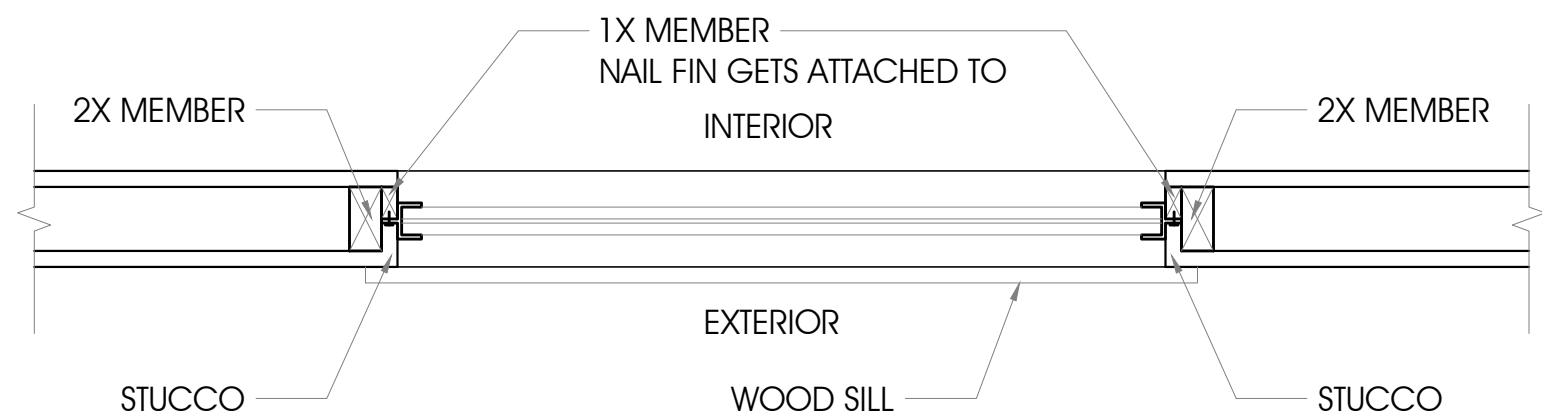
2 WINDOW PLAN DET (TYP.) Scale: 1":1'-0"
