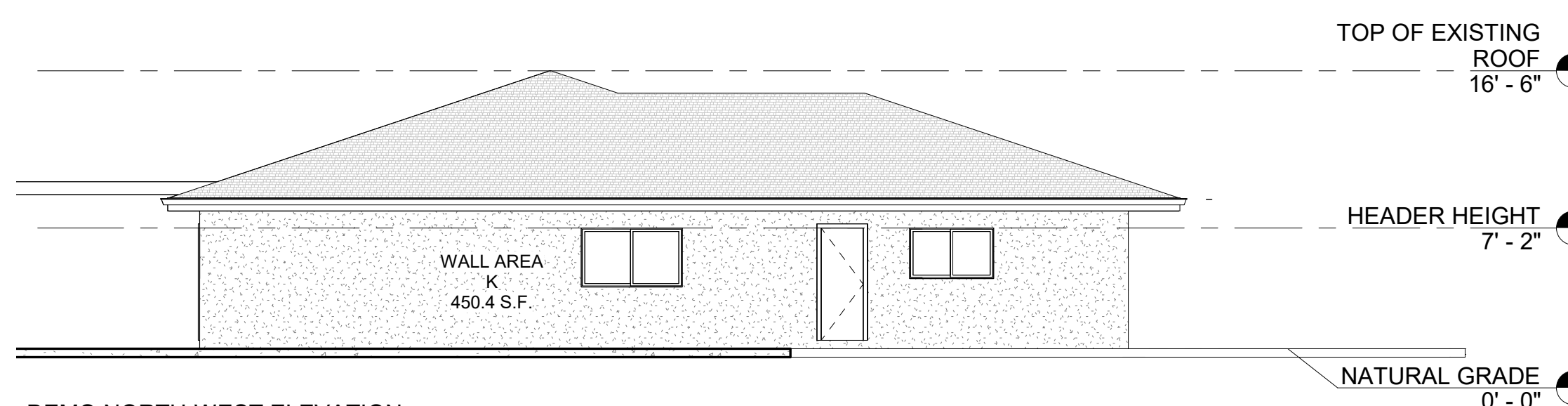
4 DEMO NORTH-WEST ELEVATION 1/8" = 1'-0"
