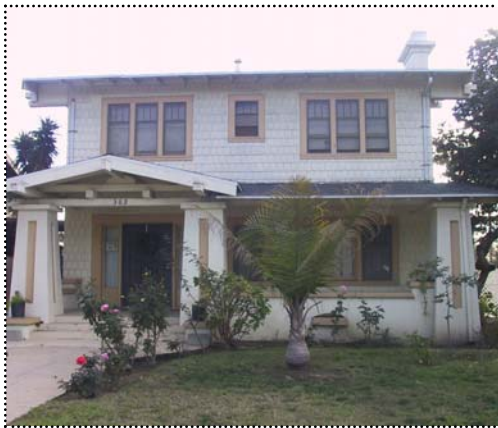
Below: While siding varied among Craftsman style houses, the wood shingle siding of this particular example is considered character-defining.
