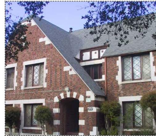
Above: This large scale apartment building uses a variety of roof shapes, dormers, changes in material and fenestration to break up the massing and to convey the Tudor characteristics.
