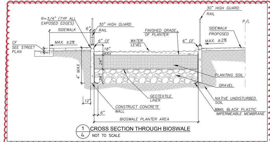
1 CROSS SECTION THROUGH BIOSWALE
