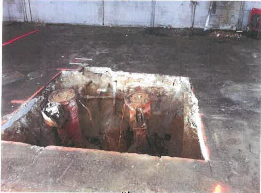
Photograph 3: View of dual post lift in Bay 27 prior to removal.
