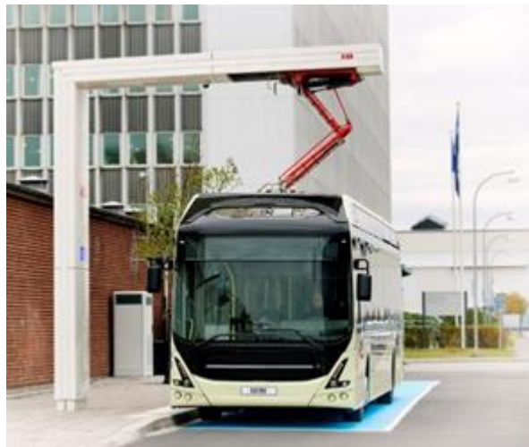
Figure 1-9: On-route Overhead Charging (Source: ABB)
