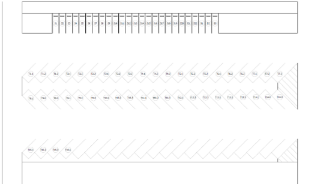
Figure 1. Option 1 Conceptual Site Plan. “S” denotes shuttle bus charging stalls and “T” transit bus.
