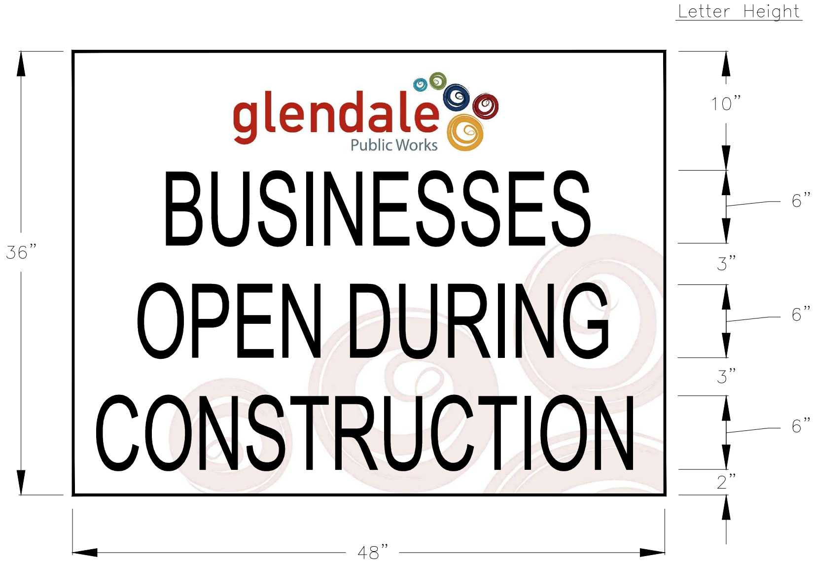
3' (36" x 48") Project Sign - Black/Red Letters on White Background with Red Logo Effects
